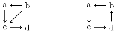
Figure 3: An acyclic and a cyclic graph for vertex set \{a, b, c, d\} . For each cluster of vertices C where |C| > 1 let f(C) be the number of vertices in C who have no parents in C (i.e. the LHS of (3)). Abbreviating e.g. \{a, b\} to ab , for the left-hand graph we have: f(ab) = 1, f(ac) = 1, f(ad) = 2, f(bc) = 1, f(bd) = 2, f(cd) = 1, f(abc) = 1, f(abd) = 2, f(acd) = 1, f(bcd) = 1 and f(abcd) = 1 . For the right-hand graph we have: f(ab) = 1, f(ac) = 1, f(ad) = 2, f(bc) = 2, f(bd) = 1, f(cd) = 1, f(abc) = 1, f(abd) = 1, f(acd) = 1, f(bcd) = 1 and f(abcd) = 0 . The cluster constraint for cluster \{a, b, c, d\} is violated by the right-hand graph since these vertices form a cycle.
