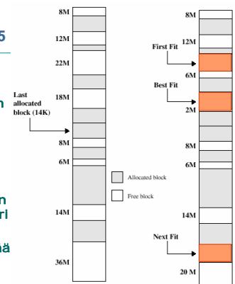
Example Memory Configuration Before and After Allocation of 16 Mbyte Block
