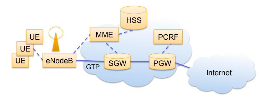
GTP: GPRS Tunneling Protocol for IP-over-UDP control and data MME: Mobile Management Entity SGW: Serving Gateway: forwards user traffic and mobility anchor PGW: Packet Data Network Gateway: external networks and billing HSS: Home Subscriber Service PCRF: Policy Charging and Rules Function
